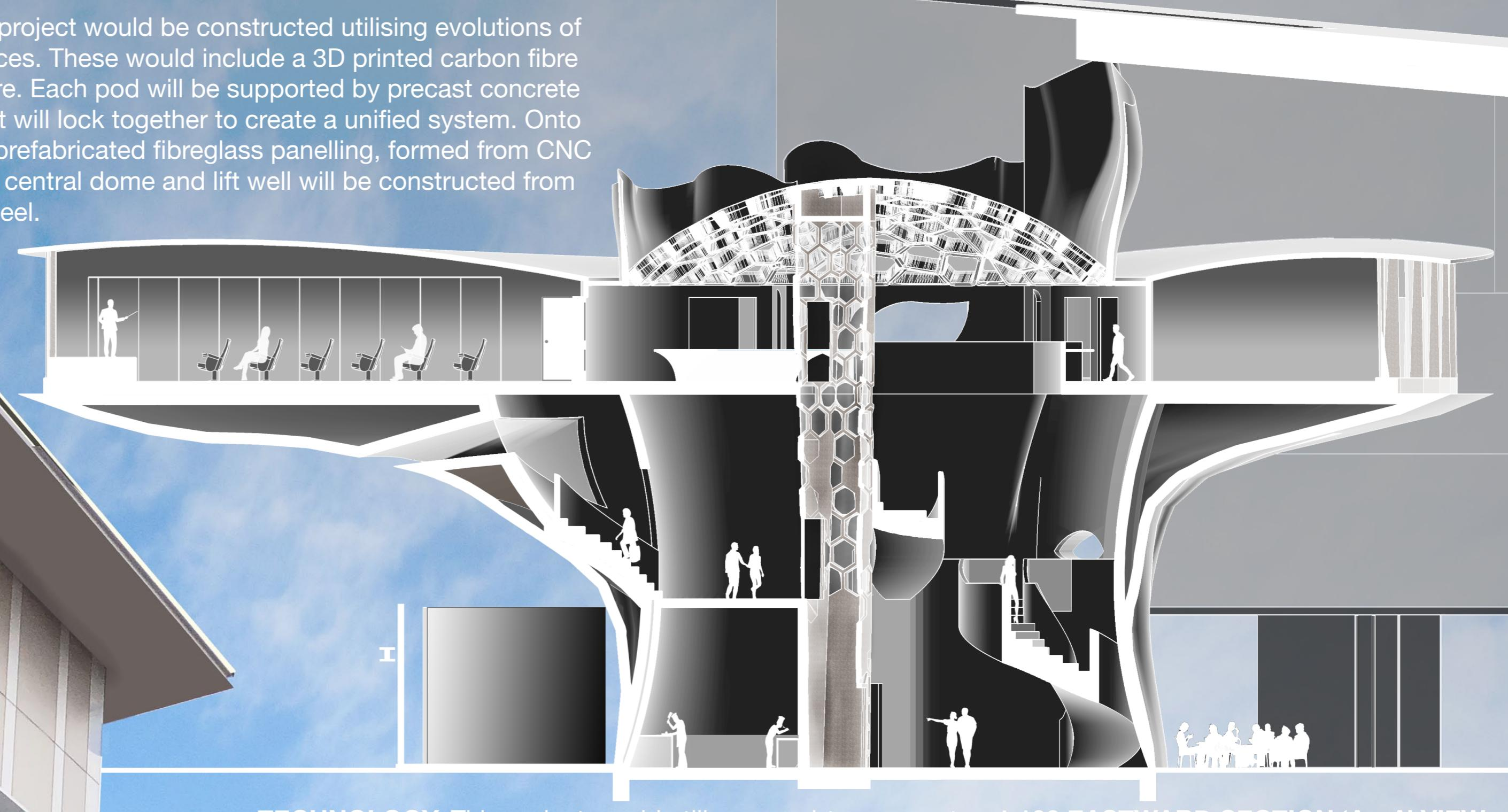
**TECHNOLOGY:** This project would utilise a semi-transparent photovoltaic film, applied to the roof and petal structures to create a unified solar panel. A Photochromic film would be applied to the ceiling glass of the central dome to reduce the penetration of direct sunlight, reducing heat gain but maintaining natural light when the sun is at low angles.
